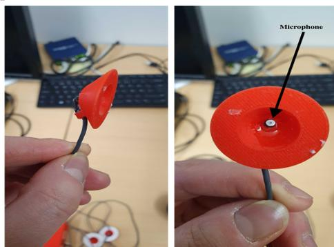
Figure 1: Cup-shaped microphones.
